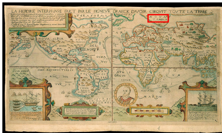
Figure 12. The Dutch-Drake 1594, La Heroike Interprinse . . . world map with Nova Zembla labelled as a peninsula of one of the great circumpolar islands. Note: This map has a prominent equator and central meridian. Each of these is linearly graduated and labelled in degrees. This confirms that the map uses an equirectangular map projection.
