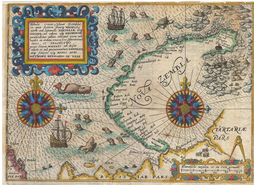
Figure 8. Nova Zembla is an island on De Veer's 1601 Tabula terrae Novae Zemblaë map. It shows their escape route of 1597. The latitude scale on the left side and the horizontal distance scale with calipers are both linear indicating an equirectangular map projection, and there are interconnected compass roses. Therefore, this is an equirectangular portolan latitude chart. Source: National Library of Norway ( https://urn.nb.no/URN:NBN:no-nb_digibok_2019080528003 ).
